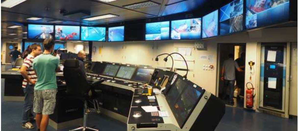
Top seen the forward navigation bridge equipped with the latest state of the art equipment including an LR DP (AAA), fully redundant Kongsberg K-Pos DP-2 and 2 x cJoy system
